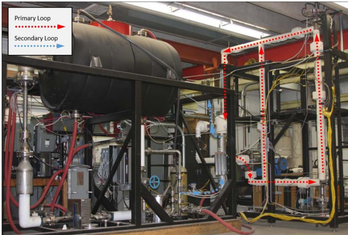
UW high-pressure heat transfer primary and secondary flow loops
